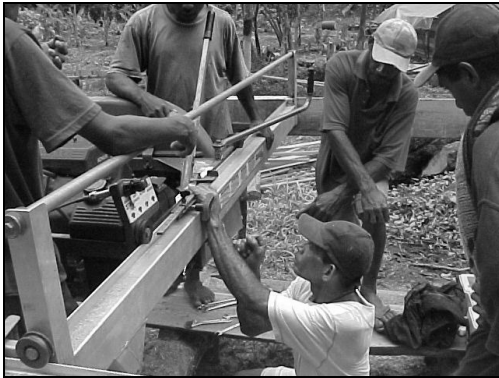
Plate 5. FPCD officer and landowners conducting maintenance on one of the mills. FPCD provides sawmilling training which covers operations and maintenance of chainsaws and sawmills.
